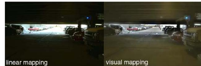
**Figure 2.** Tone-mapping of a high dynamic range image with a 10,000-to-1 intensity range. Linear mapping (left) clips the range and loses detail. The visual mapping (right) compresses the intensity range and accurately represents the scene's true appearance.
