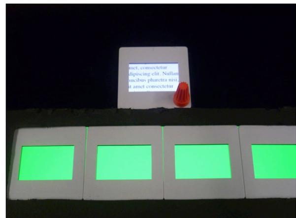
Figure 2: Setup used in the sparkle scaling experiments. Reference samples scale is along the bottom. Test sample in this case showing a text image is on the top.
