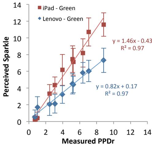
**Figure 3: Results of experiment 1 - Note the linear relationships between measured PPDr and perceived sparkle.**
