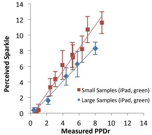
**Figure 4: Results of Experiment 2 - Note that sparkle measured using small samples is a conservative predictor of sparkle on display-sized samples.**
