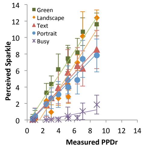
**Figure 6: Results of Experiment 3 – Note that with the exception of the “Landscape” image at high PPDr values, samples tested with real images show lower sparkle than those tested with a green screen.**
