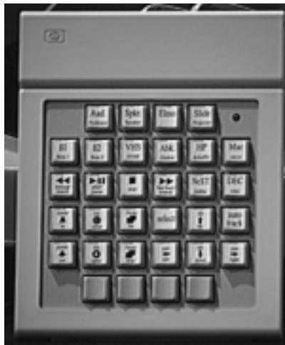
Figure 4: The Button Box. This device provides a direct physical interface to many of the same functions provided by the GUIs. The buttons can also execute macros, so complex presentation functions can be controlled by pressing a single button.
